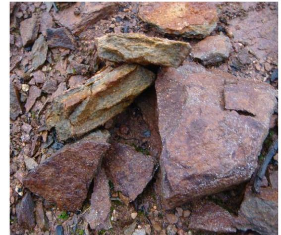
Picture of Graphitic Quartzite with about 50-70% flake graphite per volume.
